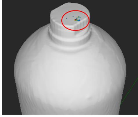
Figure 4.8: Localization of the first detected emission for the examined vessel of layup A.
