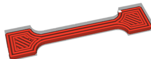
Fig. A1. Printing layer view of dog bone specimen printed by MEX method.
