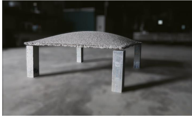
Figure 6.5: Finished squared shell prototype
