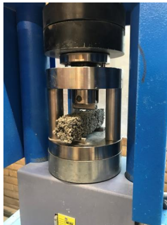
Figure 4.11: A specimen placed in the flexural test set-up and ready for testing.
