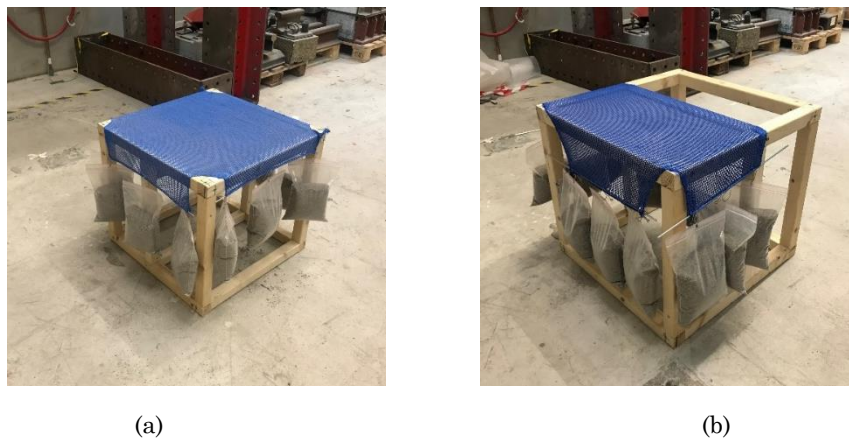
Figure 6.3: The prestressed fabrics: (a) squared geometry; (b) rectangular geometry.
