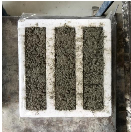
Figure 4.10: A standard sized foam mould after casting the mortar.
