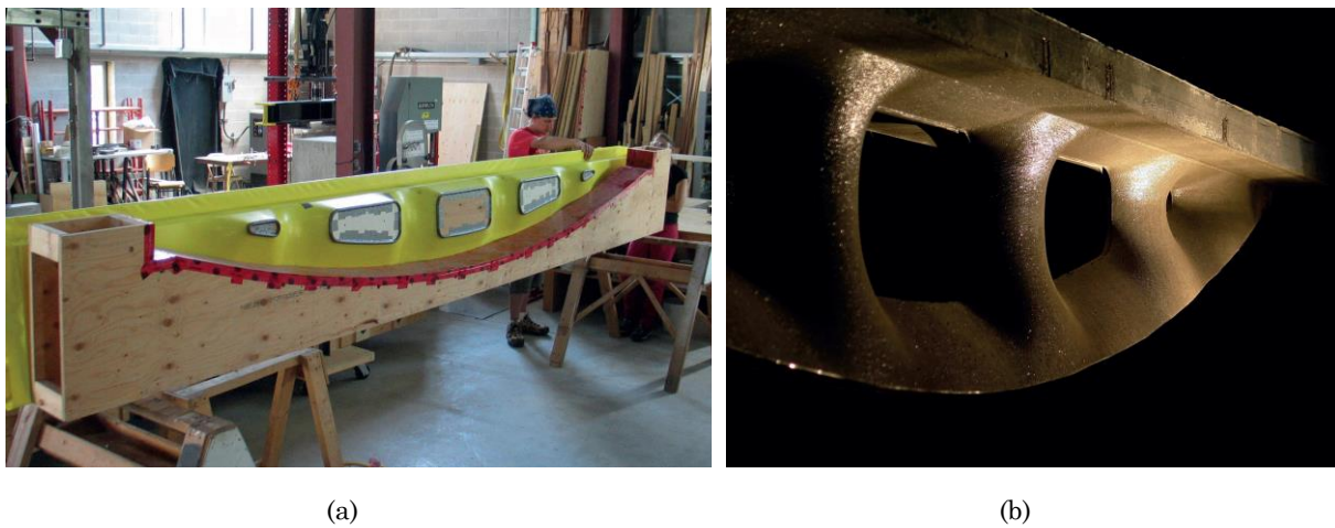
Figure 2.20: (a) Prototype mould, with a coated polyethylene fabric; (b) Prototype fabric-formed concrete truss fabricated at C.A.S.T. (photo credit: Mark West)
