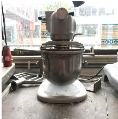
Figure 4.8: The mixer used to prepare the various mortar designs.
