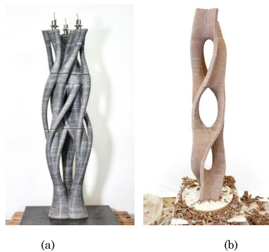
Figure 2.16: Examples of structures realised using the material extrusion 3D printing method: (a) complex shaped concrete element by Gramazio Kohler research group, Zurich, Switzerland, 2020; (b) complex shaped concrete element upon demoulding (photo credit: (a) Gramazio Kohler research group; (b) (Bruce et al., 2021))
