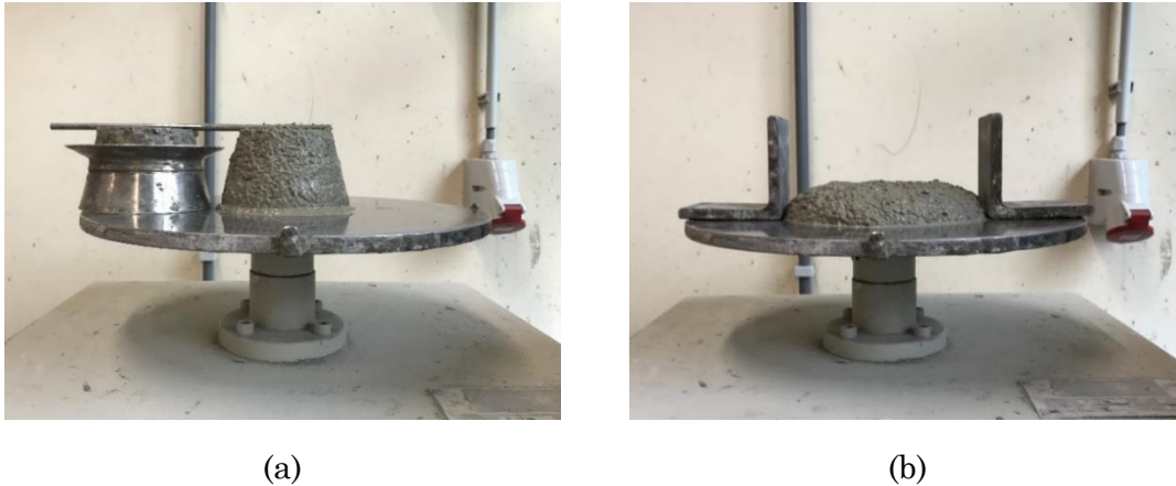
Figure 4.9: Images of: (a) the slump test; (b) the standard flow table test.
