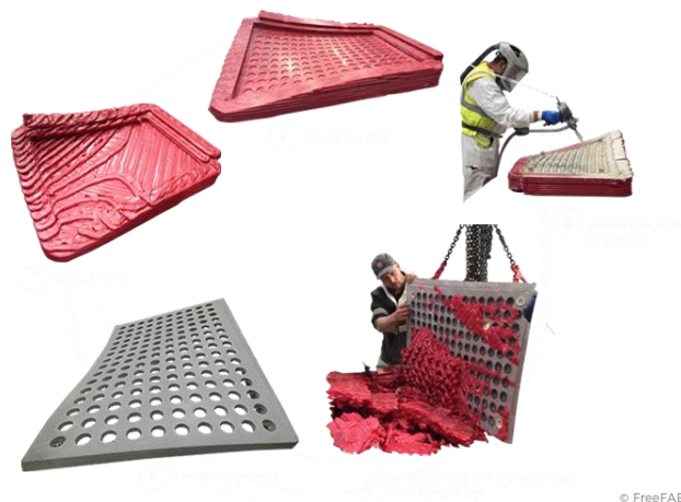
Figure 2.17: FreeFab wax moulds produced by material jetting 3D printing (FreeFAB, 2023).
