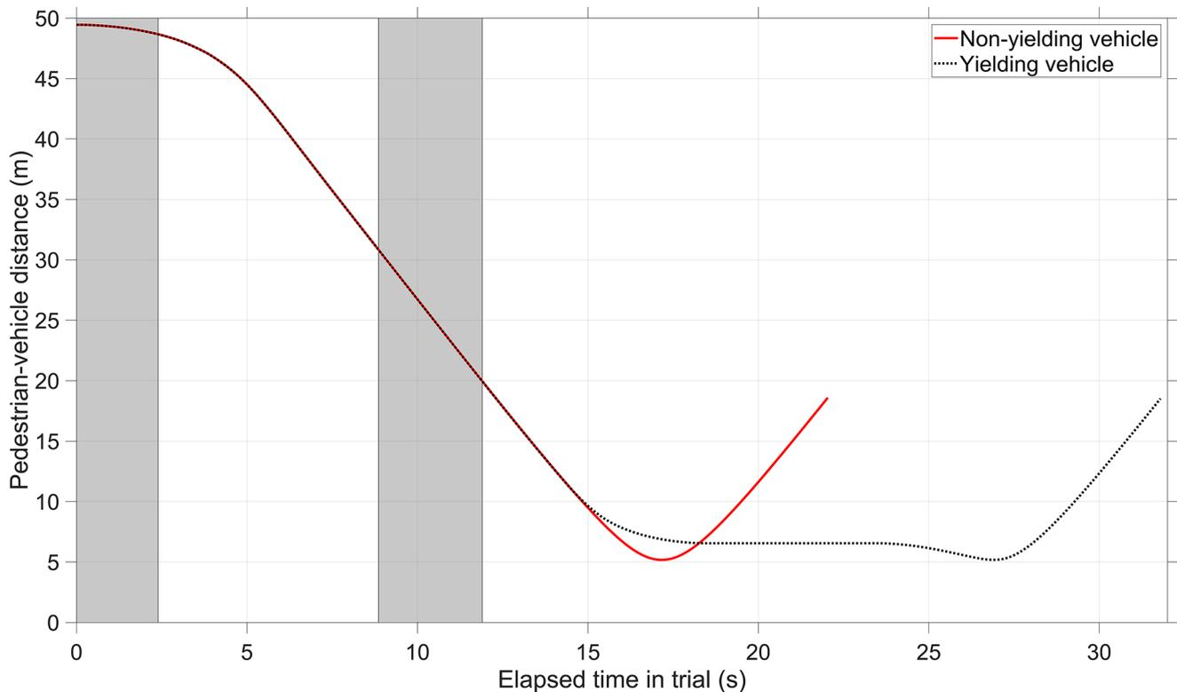
**Fig. 4** Distance between the approaching vehicle and pedestrian as a function of time. Grey backgrounds represent intervals where the vehicle could not be seen in the *Baseline* condition because it was fully occluded by the parked vehicle. Note that the yielding vehicle started to decelerate at an elapsed time of 14.3 s, came to a full stop
