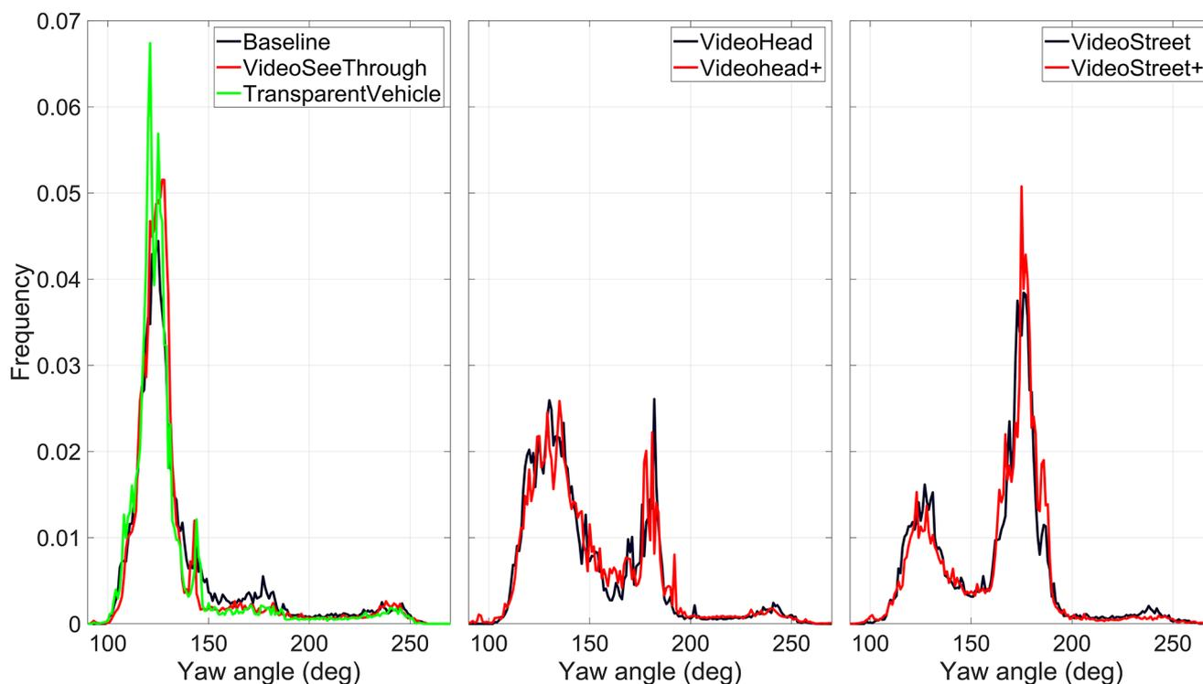
**Fig. 10** Distribution of yaw head rotation angles analysis during the vehicle’s approaching phase (0 to 14.3 s). Note that a yaw angle of 180 degrees indicates the participant gaze across the road, with angles lesser or greater than 180 degrees suggesting a leftward or rightward gaze, respectively
