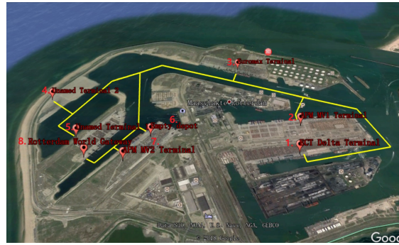
Fig. 1: ITT waterway network for waterborne AGVs in the Maasvlakte area, Port of Rotterdam from Google Earth [25].
