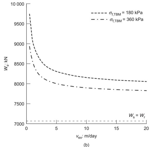
Fig. 6. Variation of  $W_s$  with (a) TBM face pressure ( $v_{ex} = 1$ – $10$  m/day) and (b) excavation rate ( $\sigma_{f,TBM} = 180, 360$  kPa)
