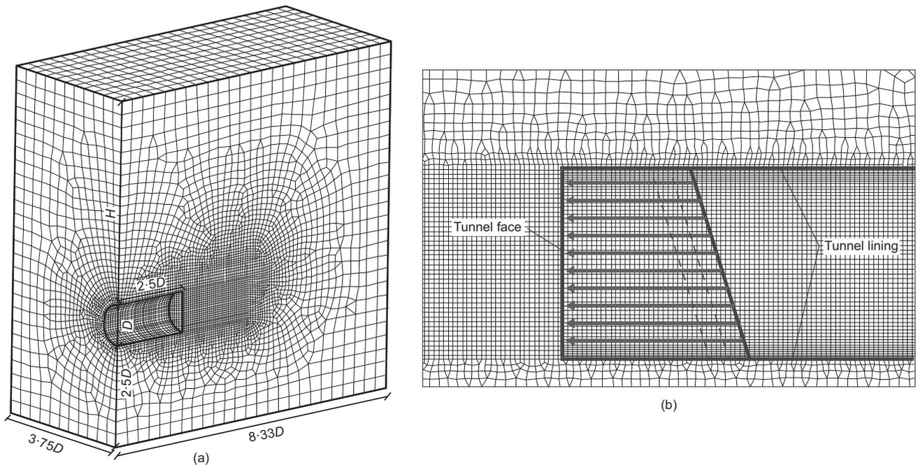
Fig. 12. (a) Numerical model and (b) progressive reduction in pressure applied at the face (adapted from di Prisco *et al.* (2018b))
