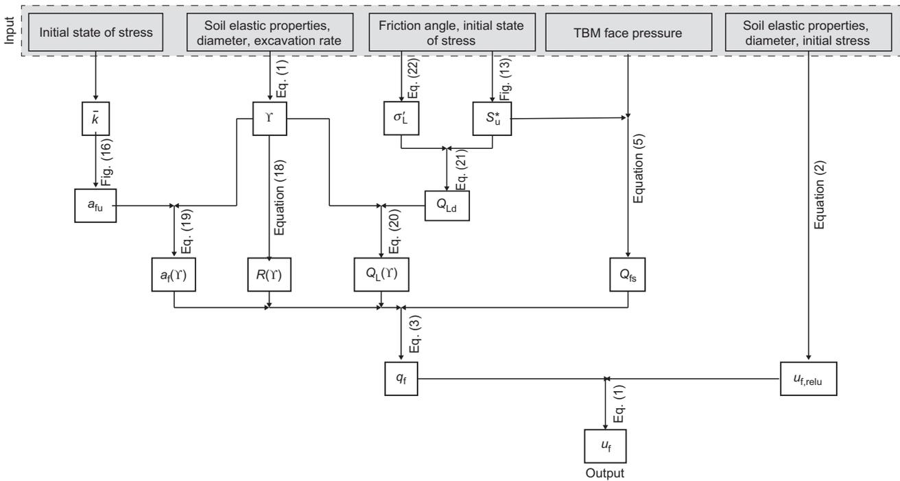
Fig. 11. Flowchart of the simplified design approach for calculating face extrusion
