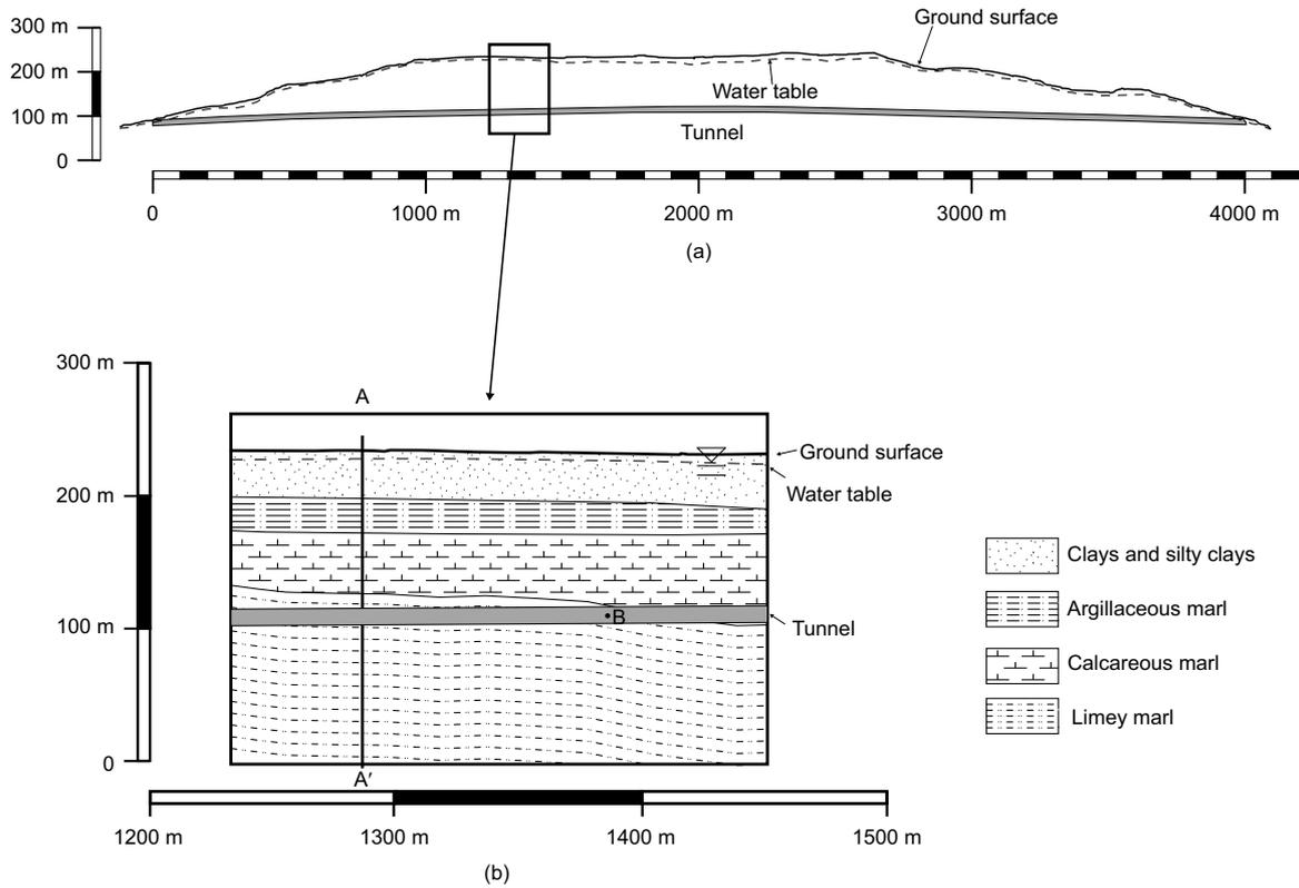
Fig. 8. (a) Sketch of the ground surface and (b) detail of the geological formations in the area of interest
