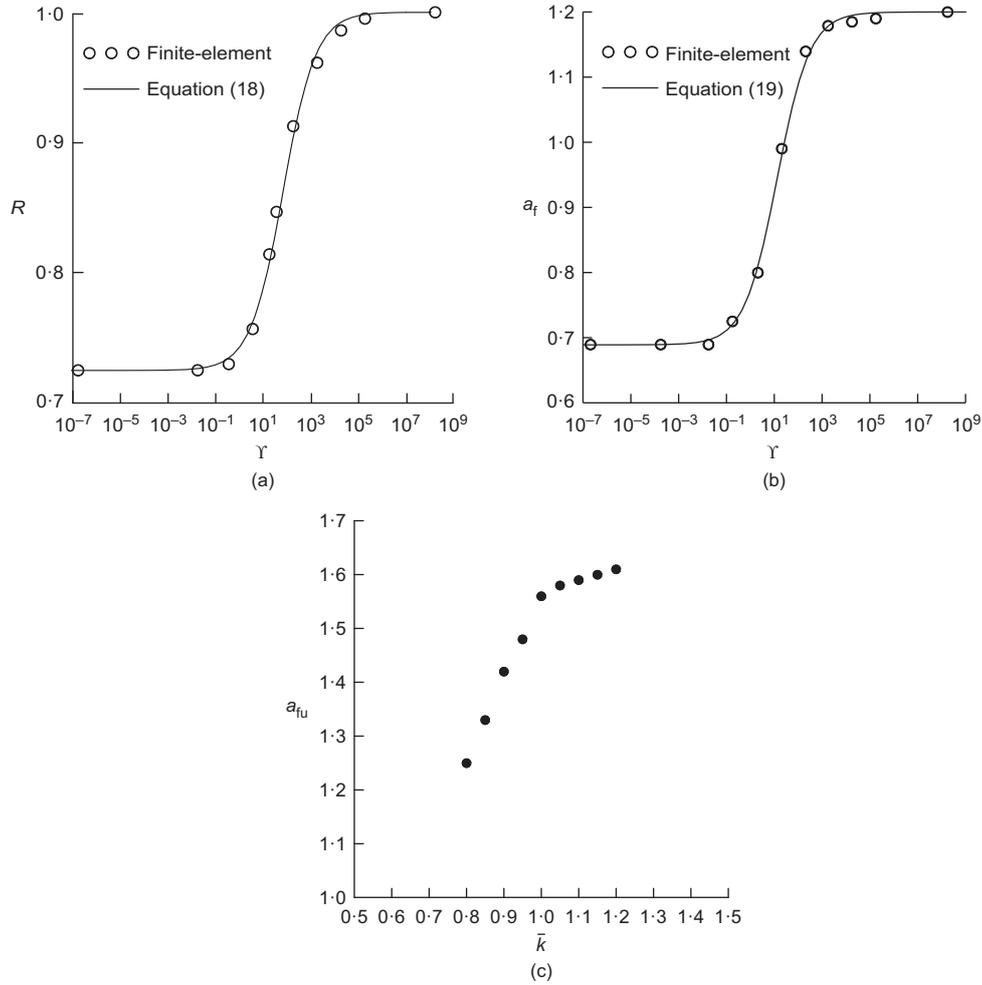
Fig. 16. (a) Variation of  $R$  with  $\Upsilon$ ; (b) variation of  $a_f$  with  $\Upsilon$ ; (c) variation of  $a_{fu}$  with  $\bar{k}$ , adapted from di Prisco *et al.* (2018b)
