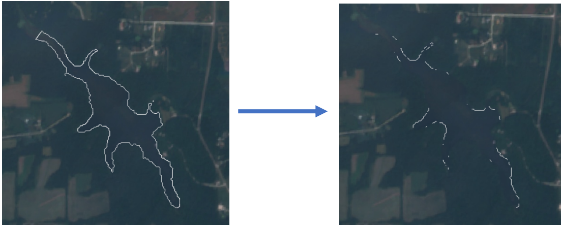
Figure 22 Effect of the slope and water occurrence noise reduction, for the construction of the water level distribution
