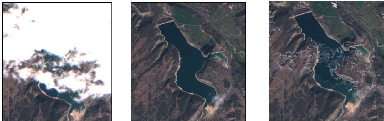
Figure 17 Cloud filtering and reconstruction of the L&R that is affected by this noise
