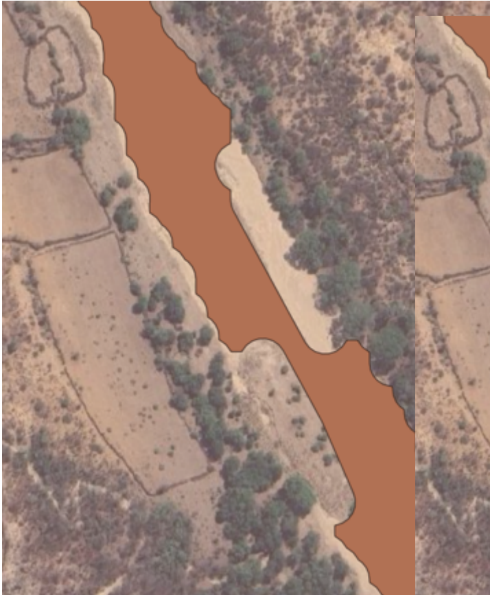
FIGURE B.6: Outcrops and vegetation cause underestimation in the delineation of the sand river. Here it is clear what to fix.
