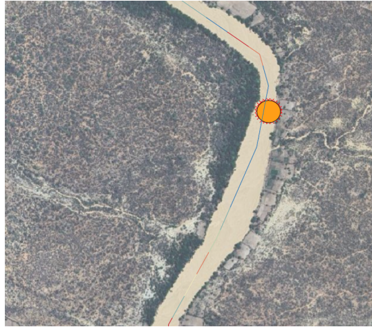
FIGURE C.33: Exception 1 with point bar and adjacent tree cover where dry season evaporation exceeds geometric water storage
