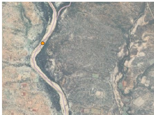
FIGURE C.34: Exception 2 with point bar and adjacent tree cover where dry season evaporation exceeds geometric water storage
