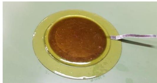
Figure 14. Dual layer epoxy sample with a 30 nm thickness gold electrode in-between layers.
