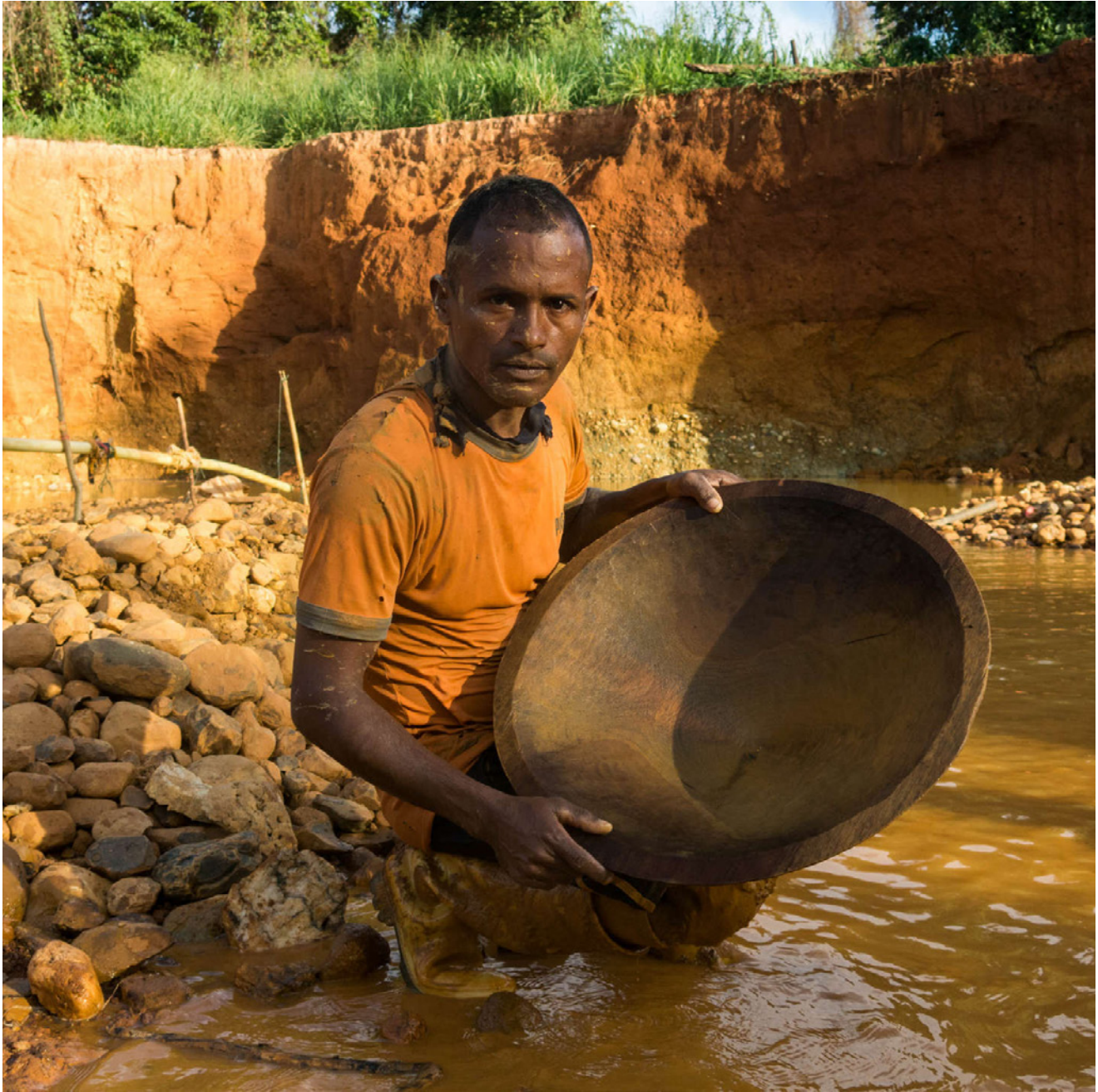
FIG. 5.3 An artisanal gold miner working in the waters of the Yuruari River, near the Nacupay sector of El Callao. Equipped with very simple and portable instruments, artisanal miners directly extract gold and diamonds from the alluvial placers of the region with rudimentary techniques. Photograph taken by Bram Ebus. Retrieved from https://arcominero.infoamazonia.org
