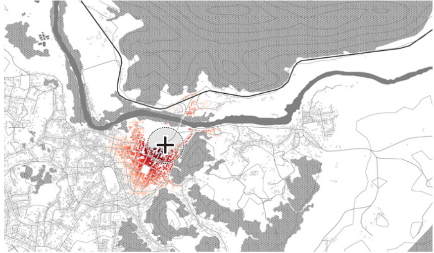
FIG. 8.36 The reach of the main passenger terminal of El Callao today, using an 800 meter radius catchment area from the station. Only the historic town center has access to the intertown transport system within a reasonable walking distance. Source: made by the author.
