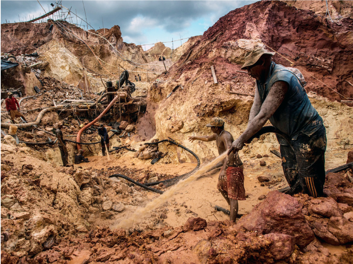
FIG. 2.25 A group of illegal small-scale miners looking for gold with hydraulic monitors at the Cuatro Muertos mine, near the village of Las Claritas. Photograph taken by Meridith Kohut. Retrieved from https://www.nytimes.com
