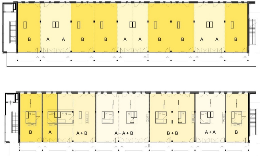
Figure 25. Load-bearing structure and permanent installations (top) Possible combinations and apartment layout (bottom)
