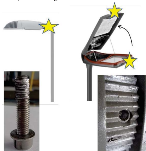
Figure 7: Overstress failure modes with spigot failure (left) and internal housing failure (right).
