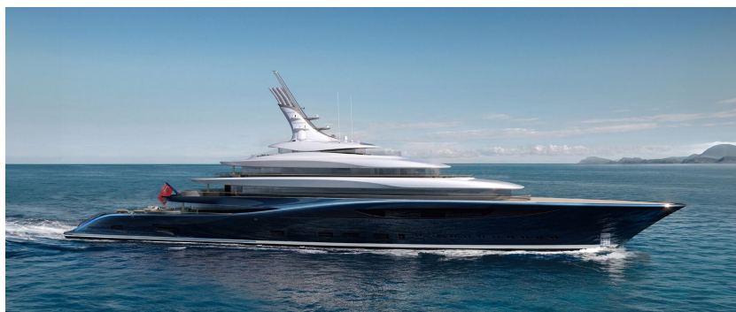
Figure 2.2: Project 821, the world's first hydrogen fuel-cell superyacht (118.8 meter), launched by Feadship in May 2024, which uses hydrogen to power its auxiliary loads at anchor.
