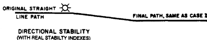
Figure 2.3: Trajectory of a directionally stable vessel, without oscillatory behaviour, [14].
