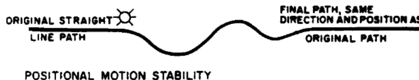
Figure 2.4: Trajectory of a vessel with positional motion stability and oscillatory behaviour, [14].
