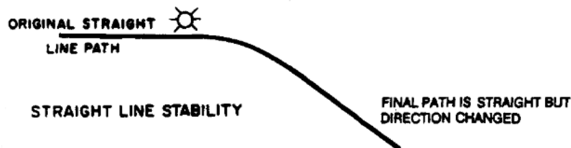
Figure 2.1: Trajectory of a course stable vessel, [14].
