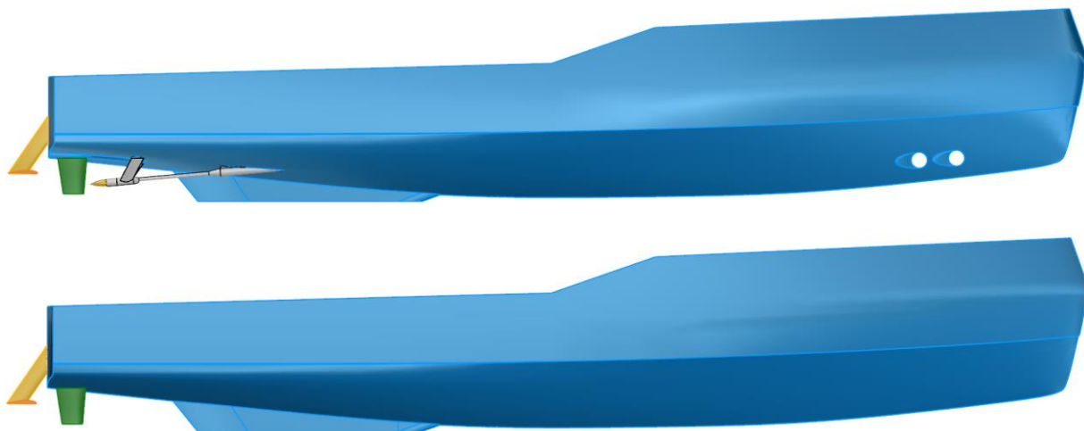
Figure 3.2: Top: Original model of RPA8 . Bottom: Simplified model of RPA8 .
