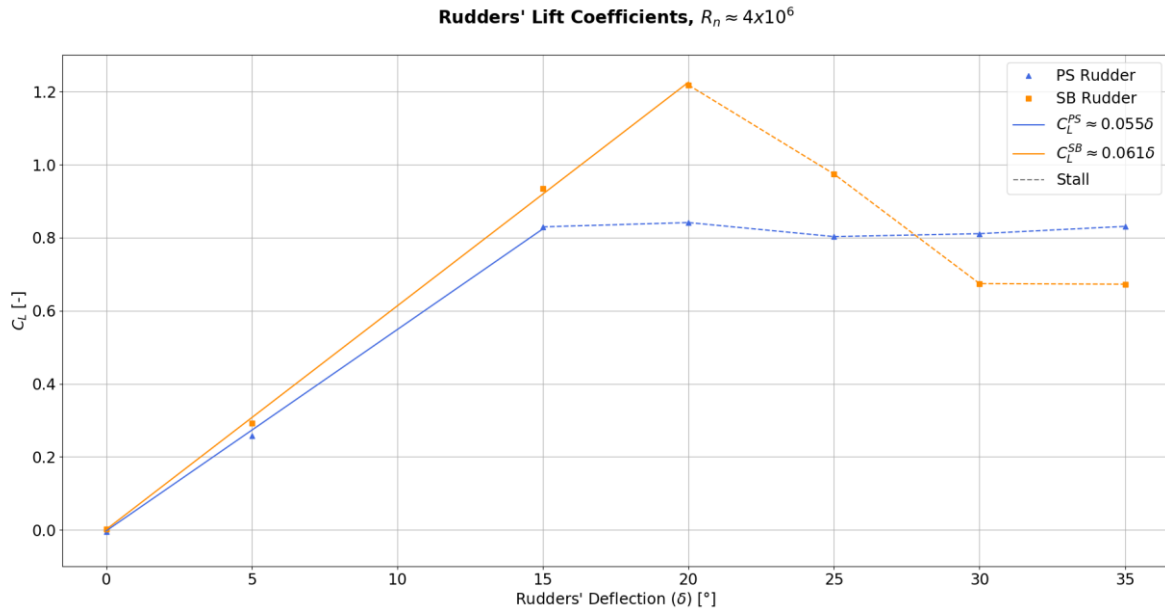
Figure 5.4: Lift coefficient curves of both rudders. The dashed line represents the after-stall region.
