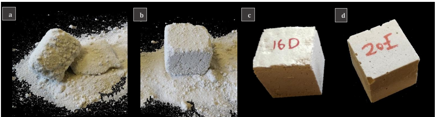
Fig. 7. CoRncrete specimen heated in convection oven with water content (a) 10%, (b) 13.33%, (c) 16.66% and (d) 20%.
