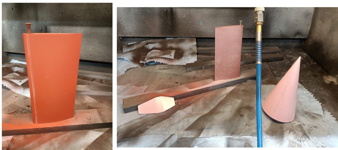
Figure 4.16: On the left: the airfoil after having been primed. On the right: the big SCB, the airfoil and the cone having been painted.
