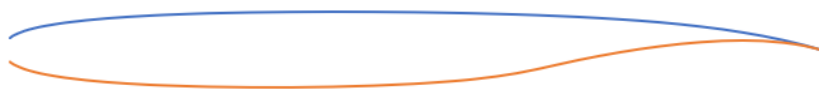
Figure 2.8: Available coordinates for 11%-thick representative NASA supercritical aerofoil. The coordinates can be found in Whitcomb (1974).
