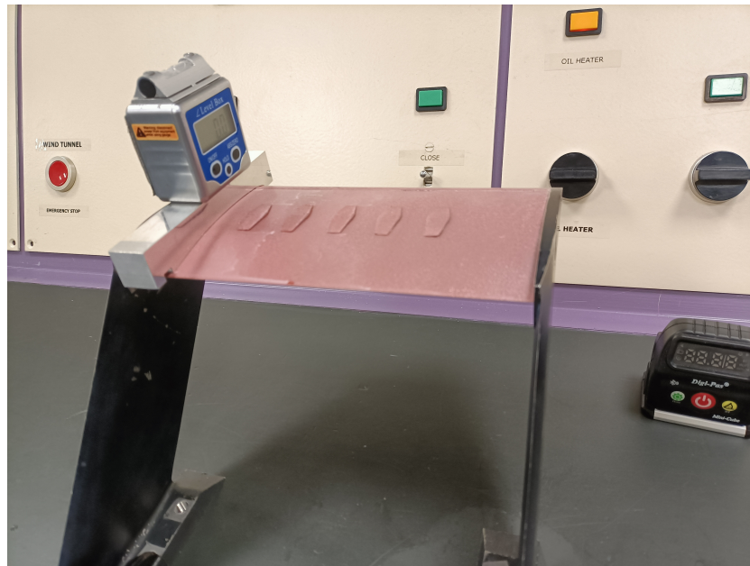
Figure 4.17: Setting the angle of attack of the airfoil.
