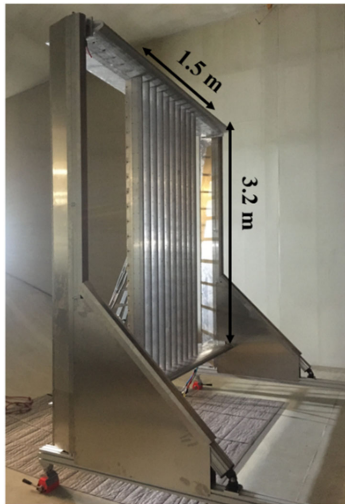
Fig. 6 Wind-tunnel seeding rake installed in the settling chamber.
