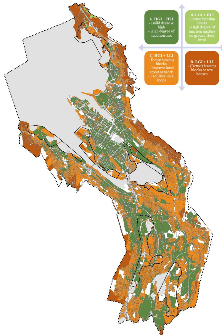
Figure 16. Strategies for where and how to densify based on the street network configuration.
