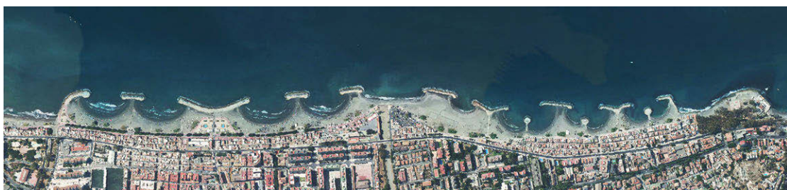
Figure 10.41: Real-life example: tomboles behind emerged (i.e. having their crests above MSL) offshore breakwaters in Malaga, Spain. Photo from SCNE ( ‘Credits’ on page 575).
