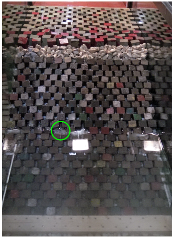
(c) Front view (one cube removed manually)
