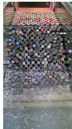
(c) Front view failure
