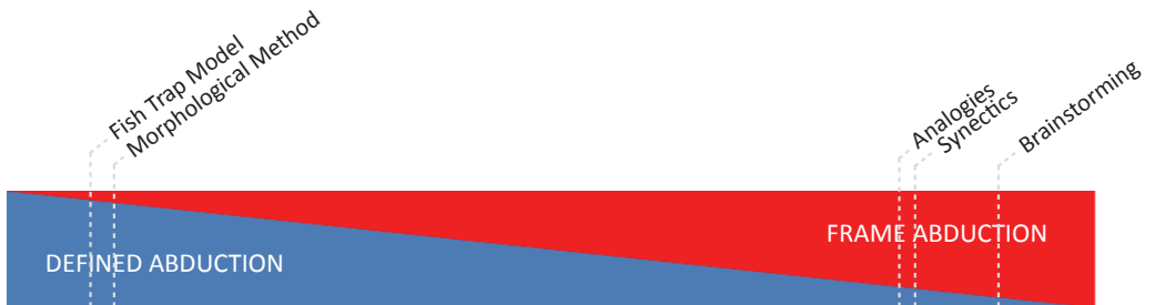
Figure 50 Modes of reasoning in design methods for framing the solution space at faculty of Industrial Design
