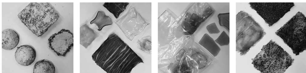
Figure 14.1 Samples from the first experimentation. From left: mycelium-based, animal gelatine-based and agar-agar-based bioplastics, damar gum and rosin, and fruit leather samples. Photographs by Stefano Parisi.
