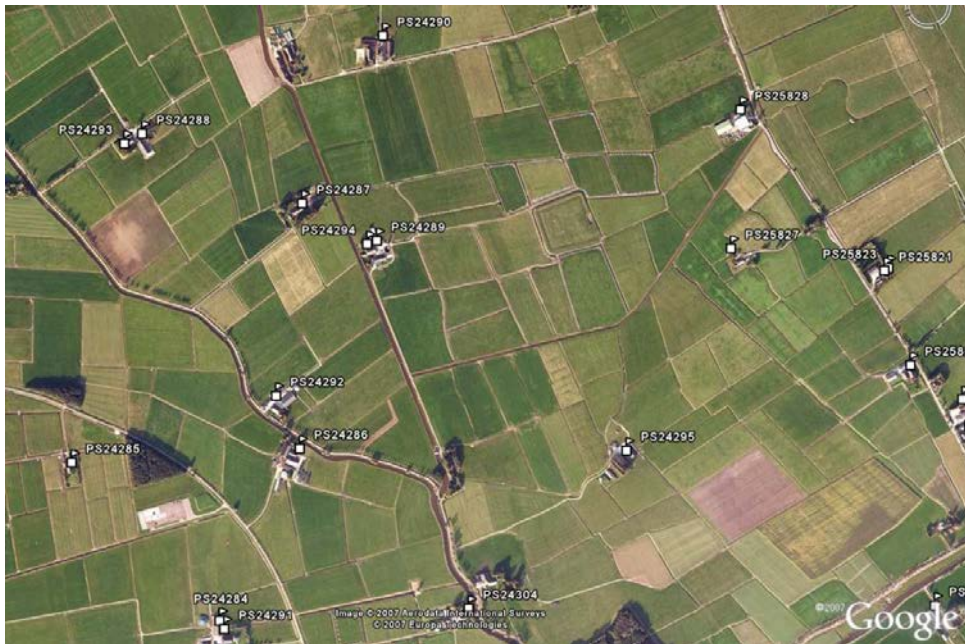
Fig. 6.12. PS targets in a rural area from four overlapping tracks (ascending, descending, and adjacent). Almost every building serves as a Persistent Scatterer.
