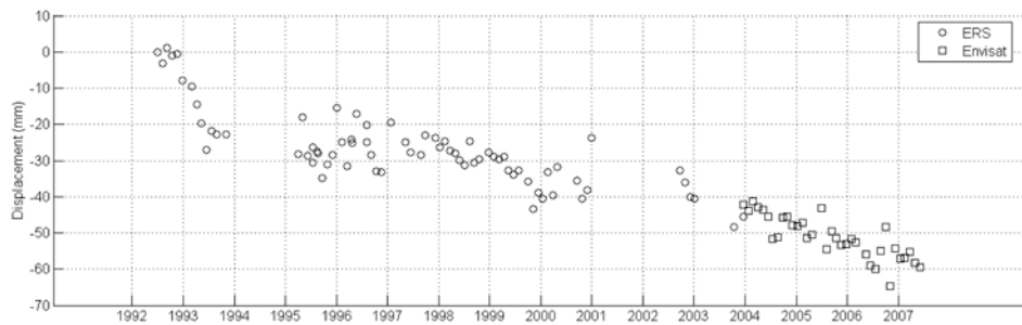
Fig. 6.16. Time series that consists of both ERS (circles) and Envisat (squares) displacement estimates. The displacement estimates have been connected in the joint estimation of a linear displacement rate.
