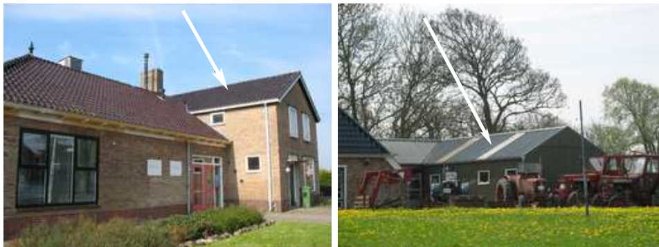
Fig. 4.22. PS targets in the Netherlands: roofs that are aligned perpendicular to the satellite look direction. These targets are most likely represented by a direct specular reflection.
