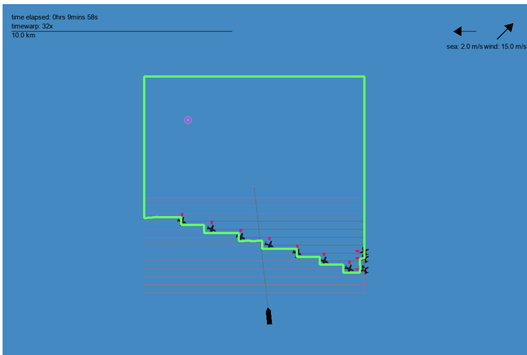
Figure 4.4: A view of the two-dimensional simulation used to analyse the swarm behaviour for the line-sweep search pattern.
