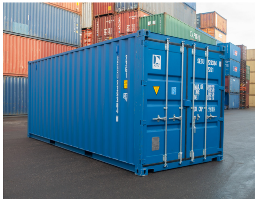
Figure 2.1: Standard 20 feet sea container [9].
