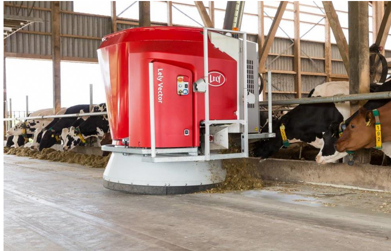
Figure 7: Lely Vector MFR feeding at the fence.
