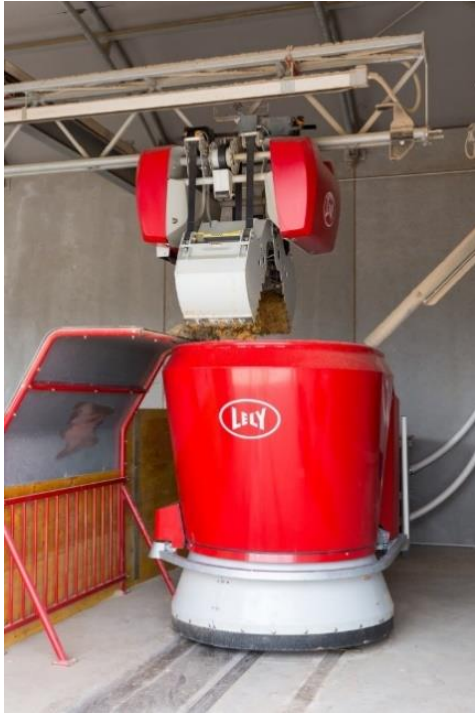
Figure 8: Lely Vector grabber and Mixing and Feeding Robot.
