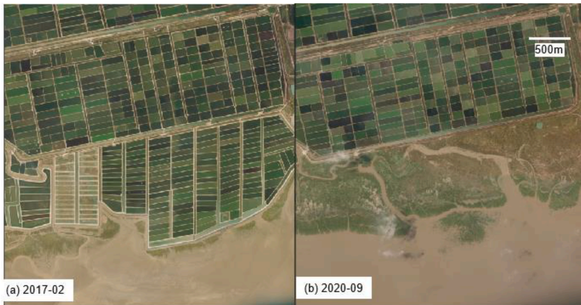
Fig. 1. Aerial view of a de-reclamation project in Jiangsu, China. (a) Reclaimed coastal area, photographed in February 2017 and (b) restored tidal flats after a de-reclamation project, photographed in September 2020. The latitude and longitude of the center of the presented area are 32^\circ 56' 06'' N and 120^\circ 54' 38'' E, respectively.
