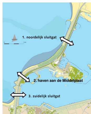
Figure C.1: Possible locations of the tidal inlet (obtained from Turlings et al. (2008))
