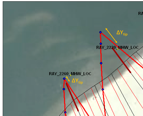
Figure G.2: Simulated accretion at the tip of two groynes when the sheltering effect for waves and currents behind groynes is accounted for in the model. \Delta Y_{tip} indicates the overestimated shoreline advance.
