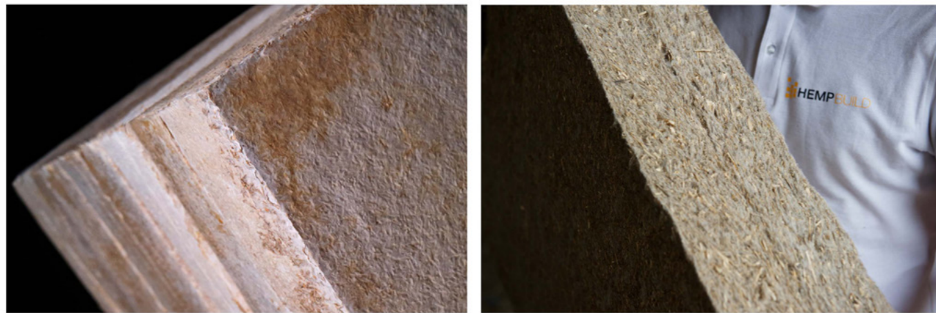
Figure 4.6 Mycelium and Hemp insulation panels (Source: Biohm, Hempbuild)
