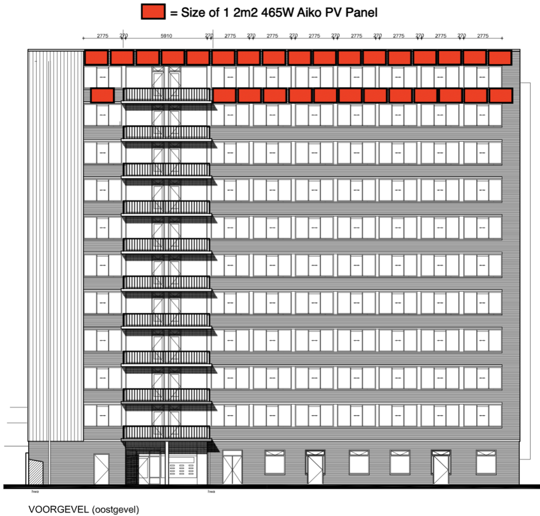
Figure 3.2. Visual of spatial estimation of 2m 2 Aiko solar panels applied to the east facing façade of the 11-story case study building, drawings from DUWO (2013).
