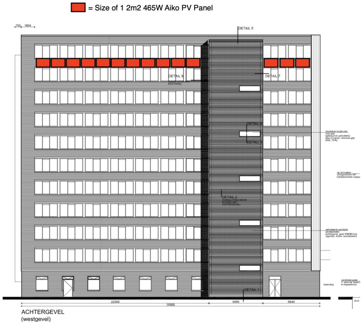
Figure 3.3. Visual of spatial estimation of 2m 2 Aiko solar panels applied to the west facing façade of the 11-story case study building, drawings from DUWO (2013).
