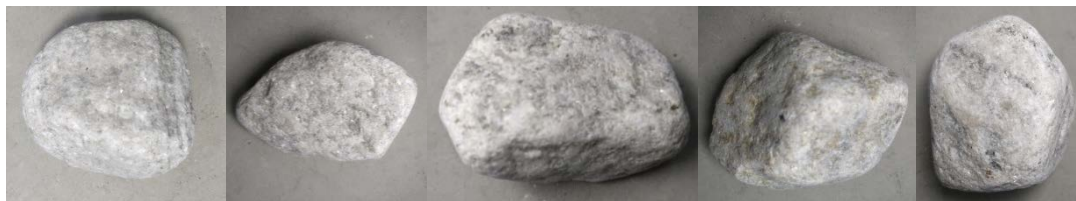
Fig.1 Recycle ballast after cleaning
