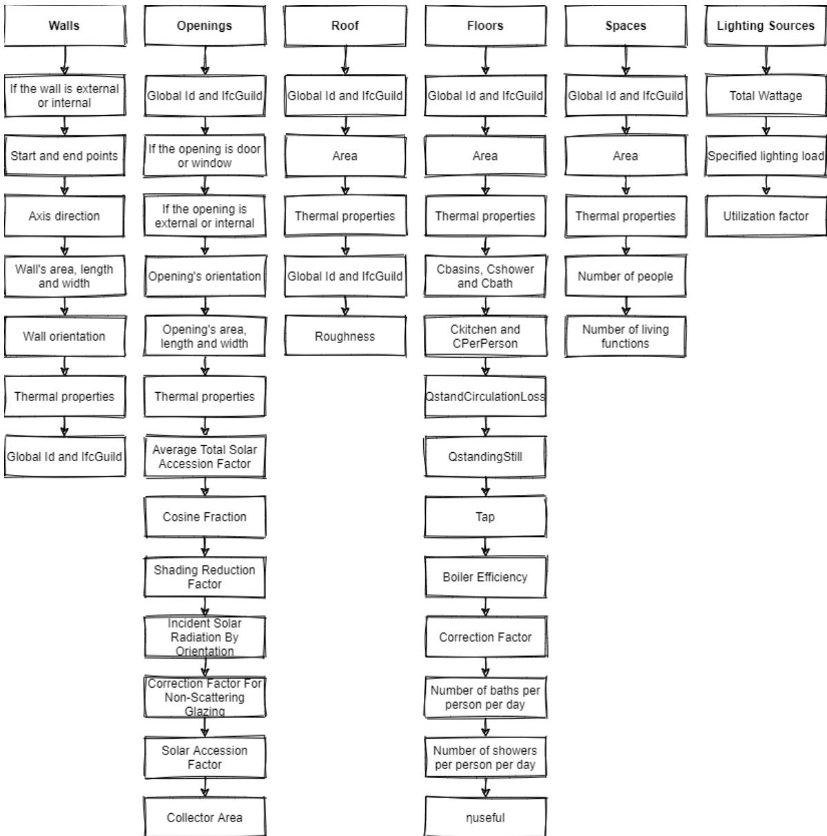
Figure 3.2: The required building data for energy calculation (Radwan 2021)
