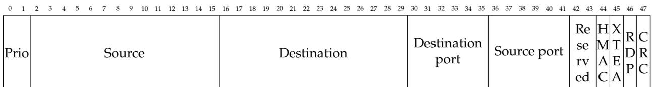
Figure 5.4: CSP version 2 header
