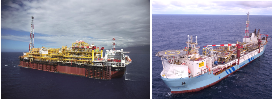
Figure 1.1: Typical FPSOs as instrumented with Structural Hull Monitoring System, both spread-moored (left) and turret-moored (right) units.
