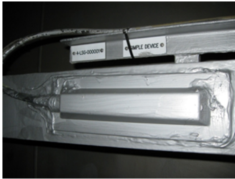
Figure 3.9: An encapsulated strain gauge after installation.
