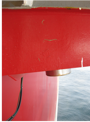
Figure 3.3: Level gauge, as mounted on the hull of an FPSO
