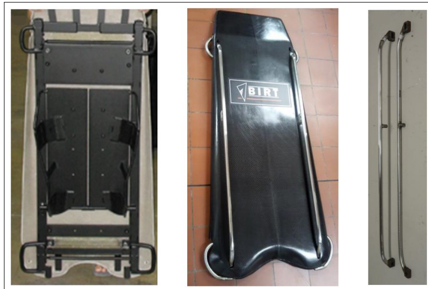
Figure A.2: The three main components of a Skeleton sled. From left to right, the frame, the bellypan and the runners. From [24]
