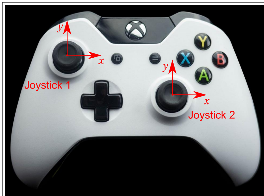
Figure 4.1: The game controller used as steering input device. The figure shows the two joysticks along with considered axes. x axis of joystick 1 acts as input for shoulder and knee steering through M_\alpha while that of joystick 2 acts as input for head steering through M_{HS} .
