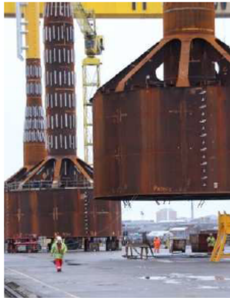
Figure 2.8: Foundation bucket concept [42].
