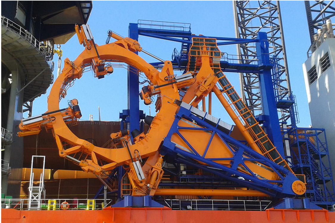
Figure 1.3: Gripper frame installed in the vessel Aeolus [1].
