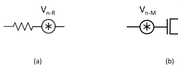
Figure B.1: (a) Noise model of a resistor (b) Noise model of a MOSFET
