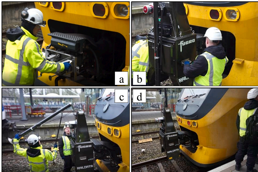
Fig. 7. Installation of mobile track inspection system: Install coupler adapter to train coupler (a); Install the measurement system to coupler adapter (b); Unfold antenna (c); Leave track (d).
