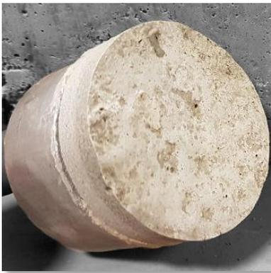
Figure 89: pulled off dolly no surface treatment
