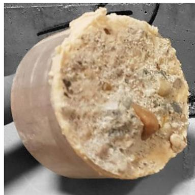
Figure 88: pulled off dolly grit blasted surface
