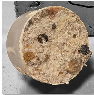
Figure 79: pulled off dolly orthogonal drilled core
