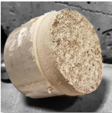
Figure 91: pulled off dolly milled surface
