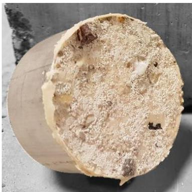
Figure 87: pulled off dolly milled surface
