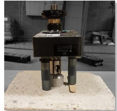
Figure 63: irregularities at the concrete surface can cause diagonal loading
