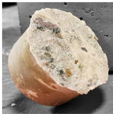
Figure 73: pulled off dolly without applying a drilled core
