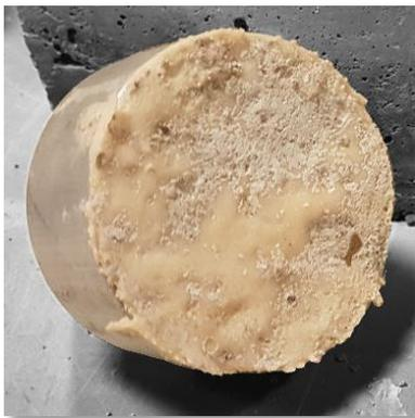
Figure 85: pulled off dolly no surface treatment
