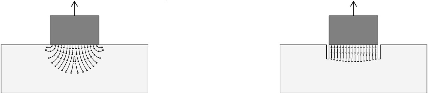
Figure 72: addressed area to distribute stresses in the situation of no drilled core (left) and a 15 mm drilled core (right)
