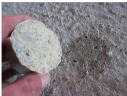
Figure 2: fracture surface after executing the Pull-Off test [2]
