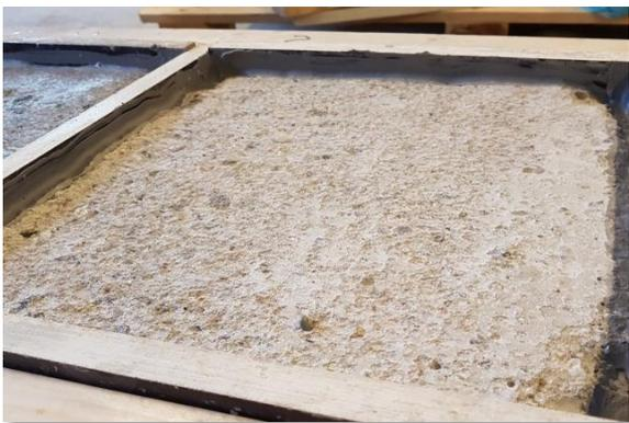
Figure 83: concrete surface treated by milling
