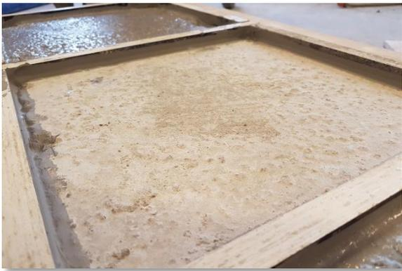
Figure 81: concrete surface not treated
