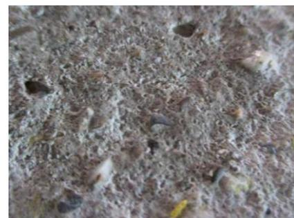
Figure 3: fracture surface on the substrate [2]
