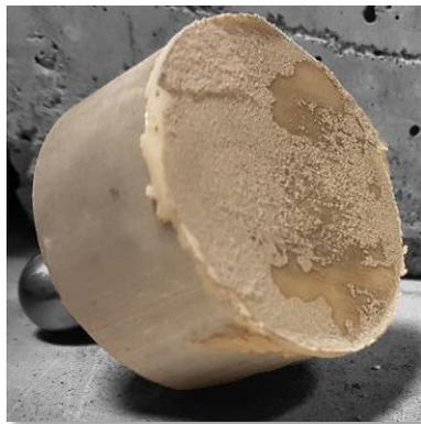
Figure 92: pulled off dolly grit blasted surface
