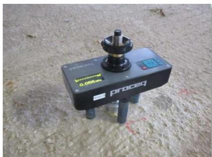
Figure 1: the automatic motorized Pull-Off bond strength tester [2]
