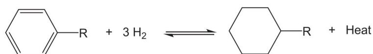
Figure 8: Systematic representation of the conversion of hydrogen to LOHC. Adapted from Reuß et al. (2017)
