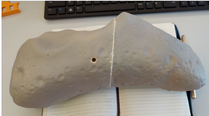
Figure 3.6: Eros10_3 after the first coat of paint, with the halves adhered together using milliput epoxy putty. The epoxy is also used to fill the gap left by the warp of the model during post-processing and to glue in the threaded insert shown.
