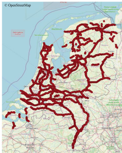
Figure 3. Geo-referenced waterway points of the shipping fleet in the Netherlands, obtained from processed data.
