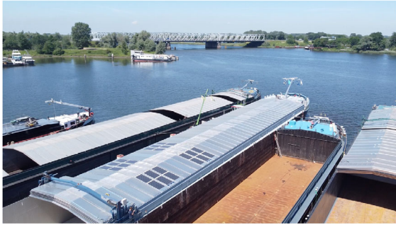
Figure 1. A bulk vessel with integrated PV. Photograph courtesy of Wattlab.nl.
