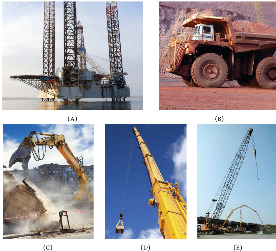
FIGURE 1.2: Applications of high strength steels in industrial structures [8] (A) jack-up oilrig legs (B) dumper-truck chassis (C) jaw crusher (D) boom of mobile cranes (E) crawler cranes
