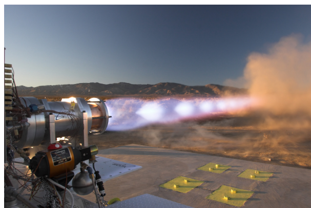
(b) Field testing of XCOR Methane rocket engine [14]
