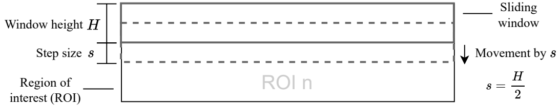
Figure 4.4: Concept of row normalization. The sliding window of height H moves with step size s . The arithmetic mean of all pixel intensities within the sliding window is calculated. Then, the mean is subtracted from all pixels within the window.
