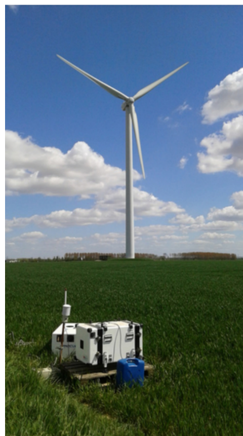
Figure 3.4: The Windcube V1 lidar with SMV6 in the background. Picture taken by ENGIE Green
