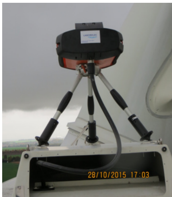
Figure 3.5: The Wind Iris nacelle lidar positioned on the turbine SMV5. Picture taken by ENGIE Green
