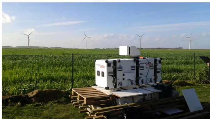
Figure 3.3: The Scanning Lidar 200S. Picture taken by ENGIE Green
