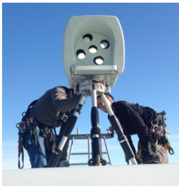
Figure 3.6: The Wind Orion nacelle lidar positioned on the turbine SMV6. Picture taken by ENGIE Green
