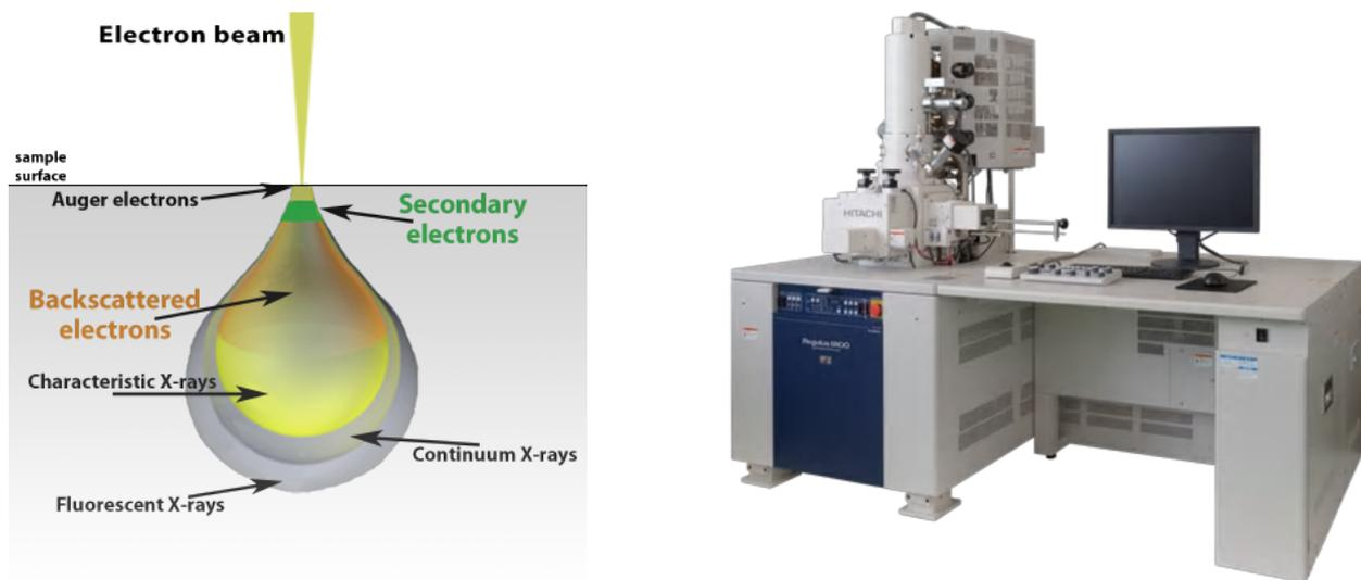
**Figure 2.15:** Left: electrons interact with solids to produce different signals[48]
