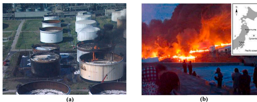
Fig. 1. Post-earthquake fires related to chemical process industry. (a) Massive fires at the TUPRAS Izmit refinery in the 1999 Kocaeli earthquake [6] (b) Oil spill fires at Kesennuma Bay in the 2011 Great East Japan Earthquake and Tsunami [8].
