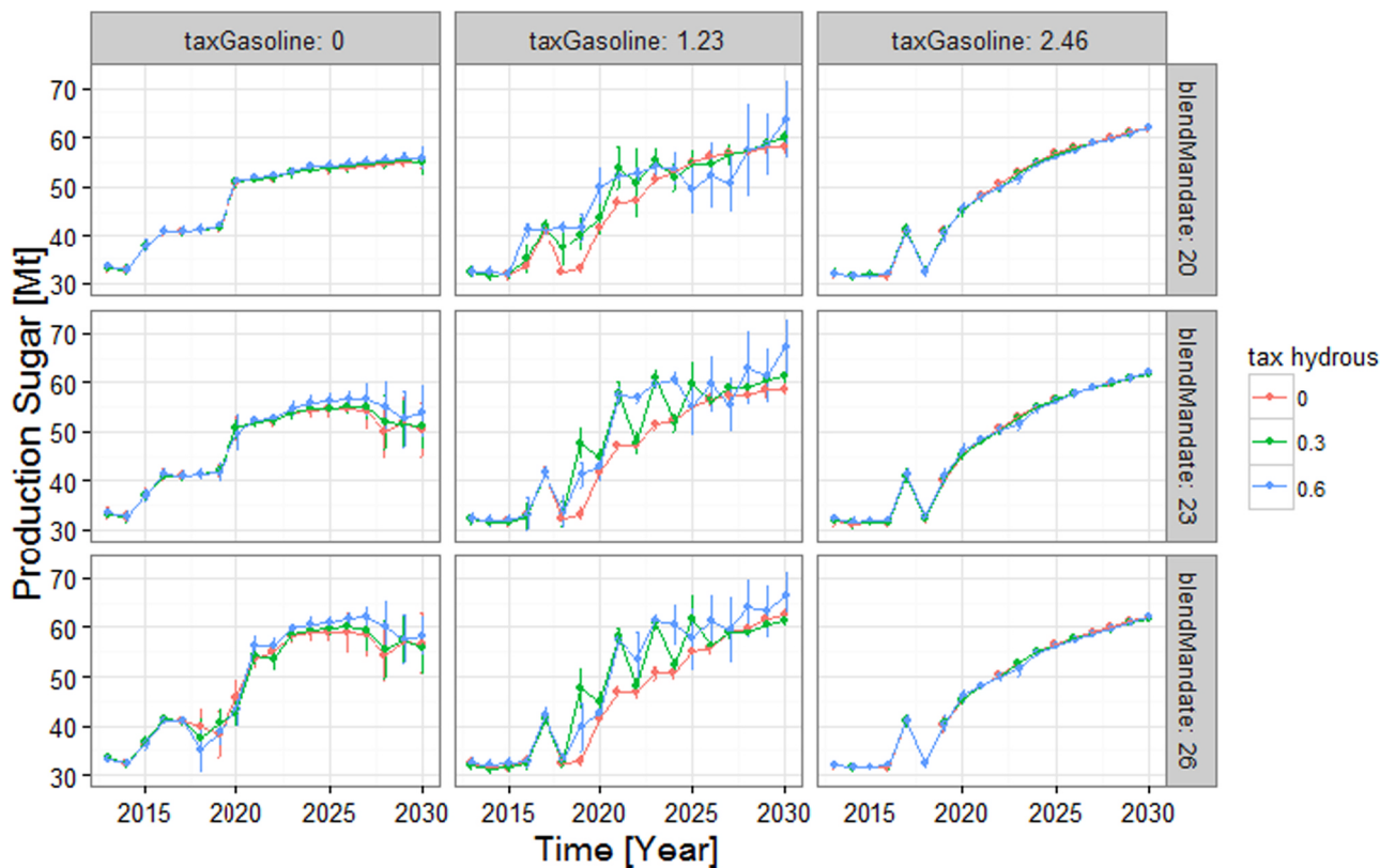
Fig. 8. Total production of sugar in Brazil over time for different combinations of blend mandate and tax levied on gasoline and hydrous ethanol. Tax on gasoline and hydrous ethanol in R$/l. Blend mandate in %v/v. Anhydrous tax = 0.05 R$/l. Dots and error bars represent the mean and the standard deviation, respectively. Forty repetitions were carried out in the simulations for each combination of policy instruments.
