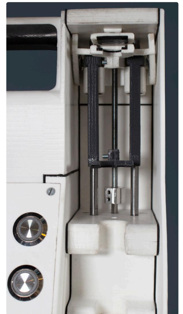
Figure I-1. The adapted syringe holder of the improved integrated fluid insertion system.
