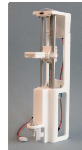
Figure F-2. The physical prototype of the initial fluid insertion system.
