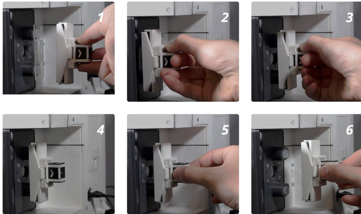
Figure K-3. Envisioned usage of removal using the improved flow cell placement tool on the integrated diagnostic setup embodiment.
