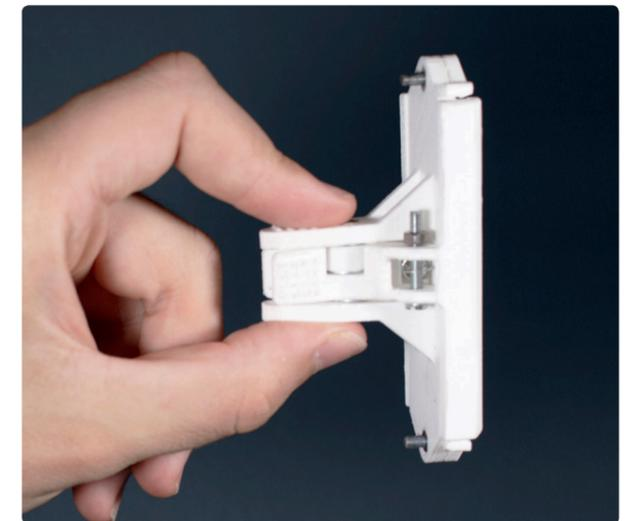
Figure J-2. The initial flow cell placement tool prototype.
