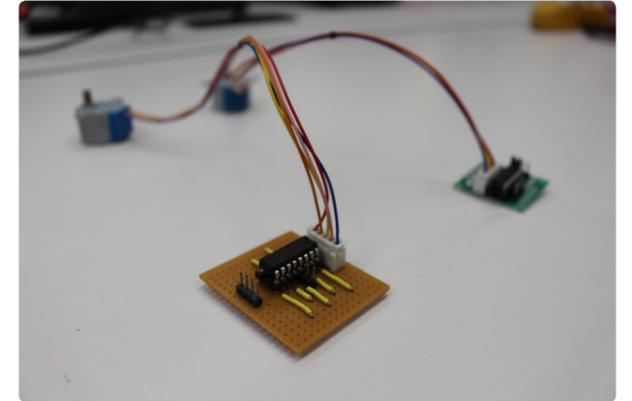
Figure G-1. Front: Custom circuit board made for housing the L293D motor driver chip connected to the bipolar 28BYJ-48. Back: ULN2003 motor driver PCB connected to the unipolar 28BYJ-48.
