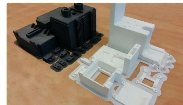
Figure E-3. Unprocessed 3D printed parts for the integrated prototype.
