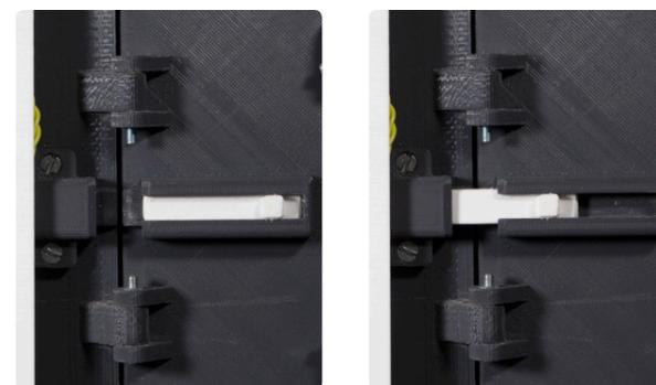
Figure E-2. 3D printed slide lock and hinge used in the integrated diagnostic embodiment.
