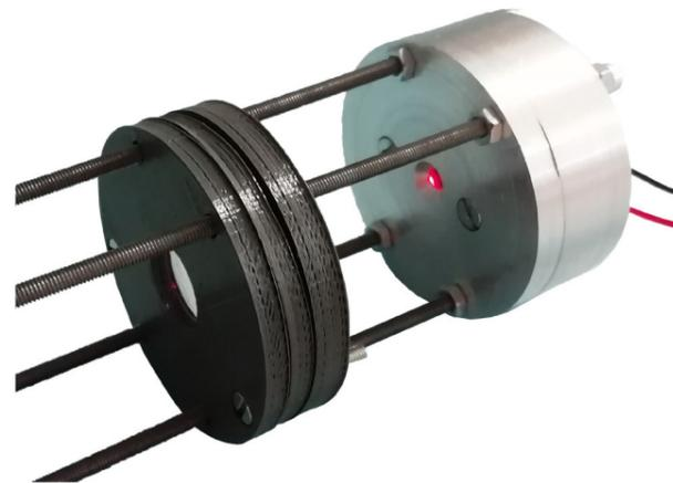
Figure D-1. Adjustable laser module frame.
