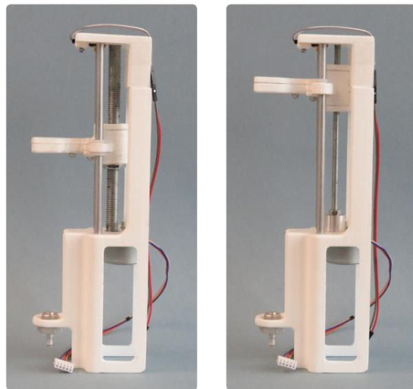
Figure G-3. Improved fluid insertion system with M10 syringe holder (Left) and M5 syringe holder (right) with according lead screw rods.
