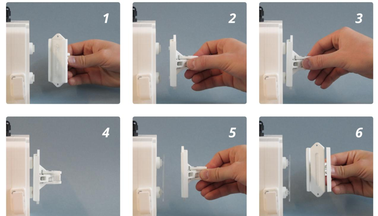
Figure J-3. Envisioned usage of the initial flow cell placement tool on the initial diagnostic setup embodiment.
