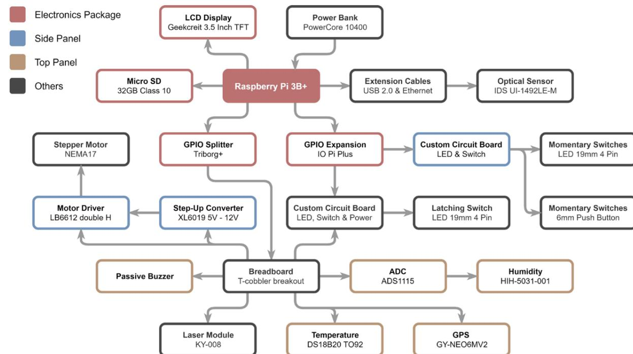
Figure P-2. Configuration of electronics in the integrated prototype with colors representing their physical location within the design.
