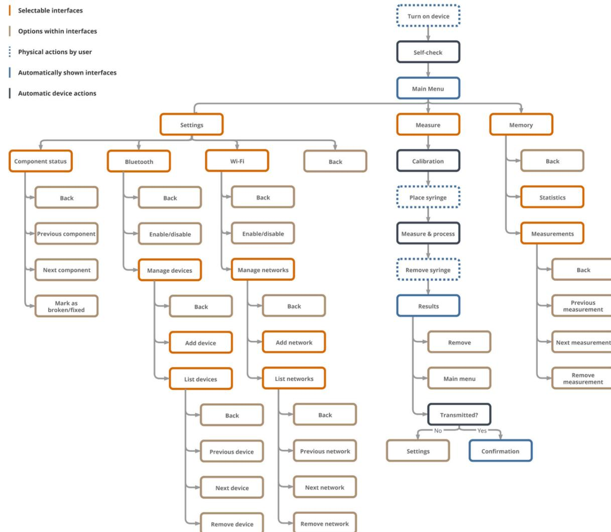
Figure N-1. Flowchart of the essential interactions for the digital interaction.
