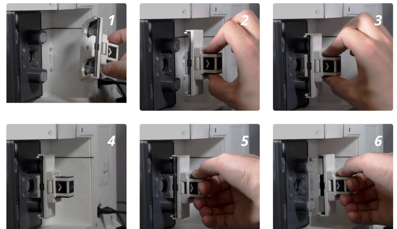
Figure K-2. Envisioned usage of placement with the improved flow cell placement tool on the integrated diagnostic setup embodiment.
