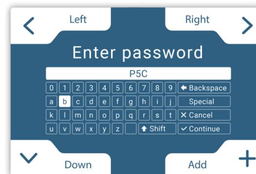
Figure O-1. The improved virtual keyboard design created for entering Wi-Fi passwords.
