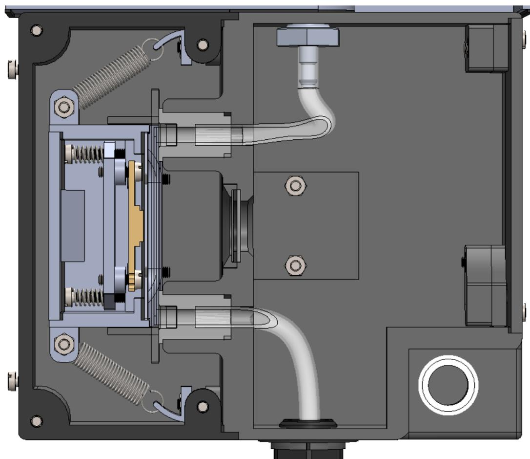
Figure E-1. Cross-sectional view of the integrated diagnostic embodiment design excluding the laser module and electronic wiring.
