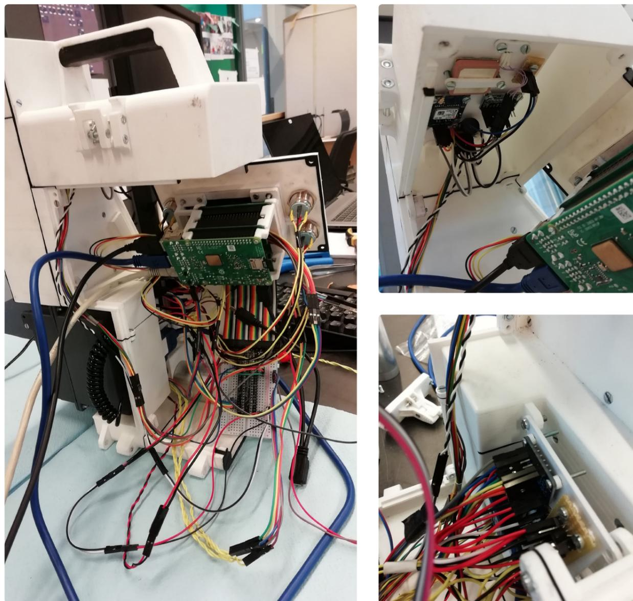
Figure P-3. Configuring the internal electronics of the integrated prototype. Left; the overall complexity of the partially assembled integrated prototype and the electronics package. Bottom right; a close-up of the side panel. Top right; a close-up of the top panel.
