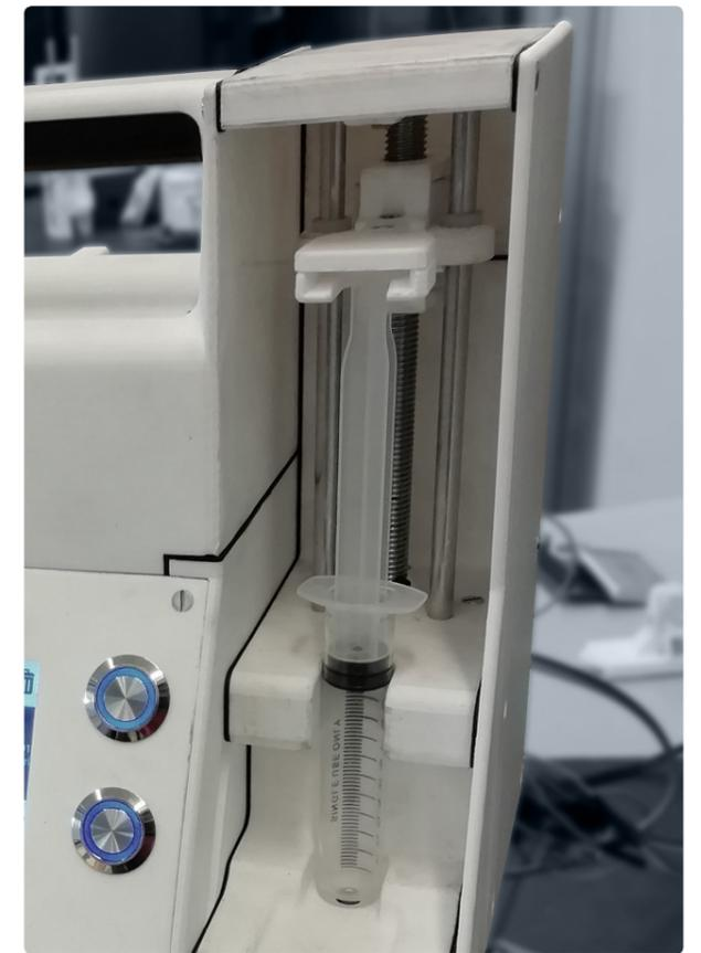
Figure H-1. Setup for validating the performance of the initial fluid insertion system.
