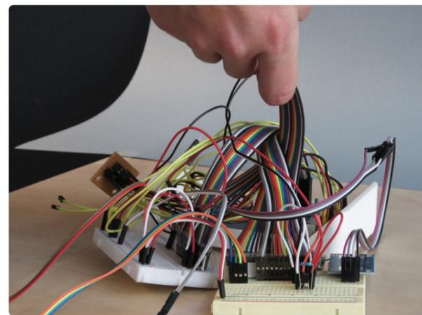
Figure P-1. Determining the desired configuration of electronics using breadboards.
