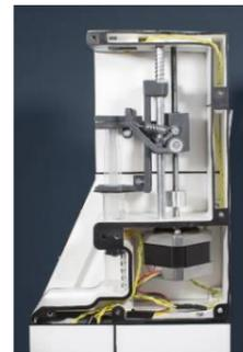
Figure 5. Fluid insertion system
