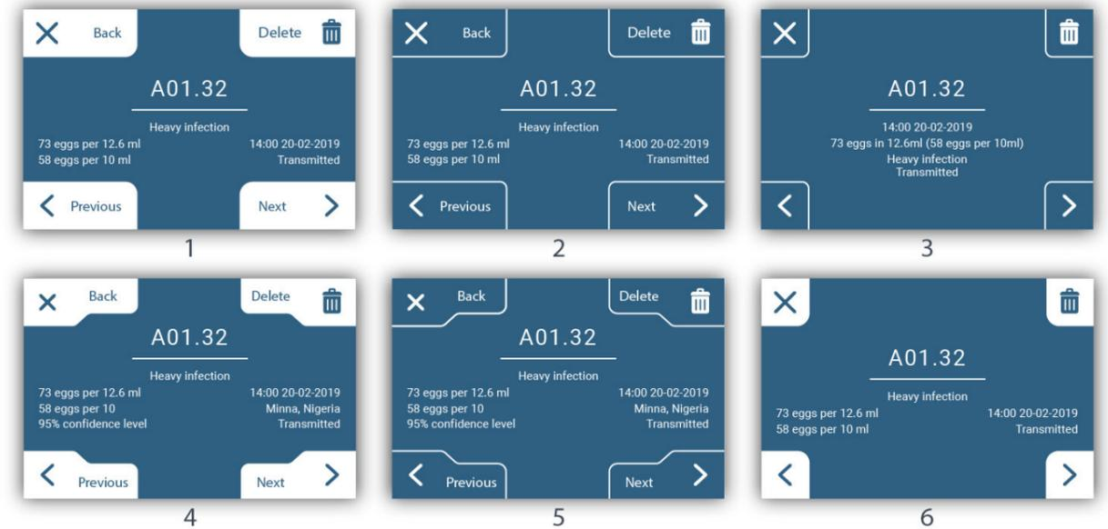
Figure N-2. General layout options for the digital interaction design.
