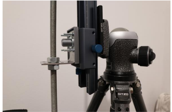
Figure 33. Zoom in picture of threaded rod to translation stage
